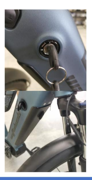
Removing the battery from the bike when storing it for a long period of time is recommended. In this case store it in a cool, dry area away from water. The charge left in the battery should be 50%-75% for long storage times.
