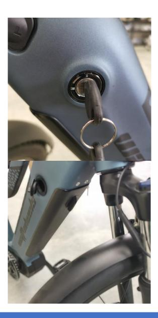
Removing the battery from the bike when storing it for a long period of time is recommended. In this case store it in a cool, dry area away from water. The charge left in the battery should be 50%-75% for long storage times.
