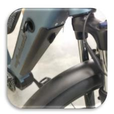
To remove the battery, turn the wheel slightly so you have better access to battery. Turn the key to the unlock position and then turn the lever on the battery case to release the battery
